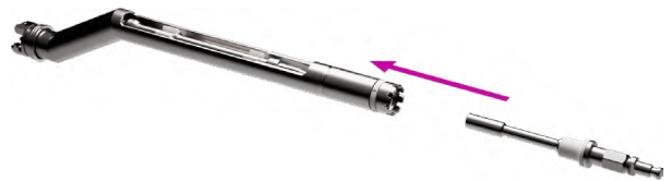
④ Insert the motor shaft into the body.
